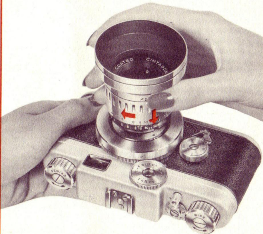
Both the Wide Angle and Telephoto accessory lenses feature ARGUS COLOR-MATIC aperture settings that may be used with average subjects in bright sunlight. The Wide Angle lens also has a Color-matic distance setting for universal sharp focus. (The Telephoto lens should be focused sharply for each picture.) Use yellow markings with Kodachrome Daylight film, red markings with Ektachrome or Anscochrome Daylight color films and with Plus-X, Supreme or similar black-and-white films (ASA 32-80).
