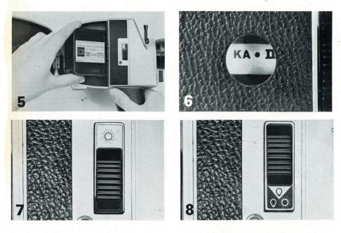
Press the cartridge into the cartridge housing also on the left side. Then the two holding springs will keep the film in the proper position. Close the cover and lock it. In loading the camera, the cartridge automatically sets the light meter for the proper film speed. A special film-type indicator window shows with what type of film the camera is loaded (ill. 6).
