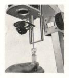
6. Attach safety filter to the shaft under the bellows.
