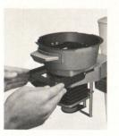
5. Insert negative carrier in position with larger tab facing upwards.
