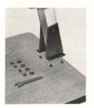
1. The baseboard holds four fixing bolts inserted halfway from its back. Screw these bolts completely so that their ends protrude rigidly from the upper surface of baseboard. Match the four holes of column to these bolts and set up the column firmly by tightening with nuts with the wrench provided.
