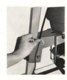
8. The line cord may be kept in position by slipping it under the clip as shown in photo 8. Mount your enlarging lens into the flange, and your 22A Special is ready for use.
