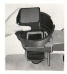
2. Place double condenser assembly in lower lamphousing and seat in the recess for it above the negative carrier opening.
