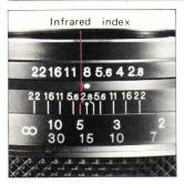
In infrared photography, some adjustment must be made in the focus in order to retain sharpness on the film, because the invisible infrared rays are longer in wave length than the visible rays used for focusing. For infrared photography —
