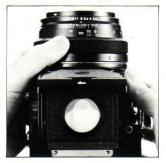
A. The lens is focused on the subject, by rotating the focusing ring in either direction, while checking the effect on the microprism / split-image range-finder spot in the center of the focusing screen (standard type).
