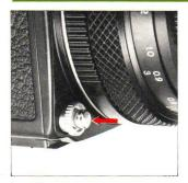
A. Depress the shutter release button with the ball of the finger. Press all the way in with a smooth and gentle action. There is no need for strength or jerky action, which will induce camera shake and affect picture sharpness.
