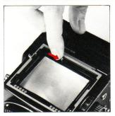
A. The focusing screen can be exchanged, depending on the type of photographic work being undertaken.
