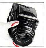
B. To attach the lens to the body, first, align the red dots on the lens and body and then insert the lens fully into its mount. Rotate in the counterclockwise direction until it stops, with an audible click which will indicate that it is securely locked.
