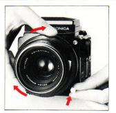
Next, while keeping the lens release button depressed, rotate the lens in the clockwise direction, too, until it makes a full stop, at which point it can be detached.
