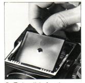
B. To install the focusing screen, insert the protrusions at the forward end of the focusing screen frame into corresponding openings in the focusing screen frame of the body. Then, drop the rear end of focusing screen and slide the screen removal lever to the right.
