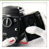
B. Depress the film back release button and the lower end of the film back can be removed, as illustrated. Simply shift the film back up slightly and pull it away.
