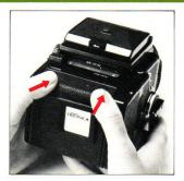
H. Close the back cover, by pressing it firmly against the base of the film back, as illustrated. The back cover will automatically lock and close, with the safety lock also locking the back cover release button.
