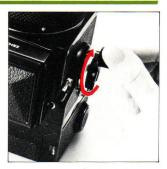
I. Upon loading the film, rotate the film winding crank until it stops to place the first frame into place for taking the picture. The exposure counter will also change from "S" to "1", while the shutter will also be cocked.
