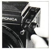
A. Always use flash cords with a standard PC type plug. When detaching the flash cord, grip the plug firmly and pull it out straight, instead of using a twisting action.
