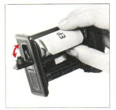
D. There are two spool holders on the film holder. The top one is for the fresh film spool while the bottom one is for the empty take-up spool. The left-side shafts of both spool holders can be opened outwards, as illustrated. Therefore, insert the right end of the spool on to the right-side shaft, which is fixed, and then close the left-side holder (shaft) which will engage the spool.
