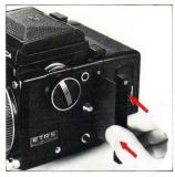
A. To remove the film back from the camera body, insert the dark slide into the dark slide slit, as illustrated, with the mark on the dark slide at the top end. Push it all the way in.
