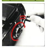
Rotating the film winding crank completely one time, in the forward direction, will advance the film one frame and, at the same time, cock the shutter, with the winding action stopping automatically. On the other hand, short, rapid strokes, up to an accumulated full rotation, will also do the job.
