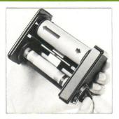
F. Unfold the manual film winder on the right side of the film holder and rotate in the arrow-indicated direction, while checking the advancing film. When the starting point, or arrow mark, is aligned with the triangular variety start-mark on the top left side of the film holder, stop rotation.
