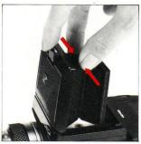
C. The magnifier can be flipped up into viewing position, by simply sliding the focusing hood/magnifier catch in the arrowindicated direction (to the left). To return the magnifier to its storage position, simply push it down until it catches.
