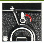
B. Upon taking the multiple-exposed picture, be sure to return the multiple exposure lever back to its vertical position and cover the red mark. Otherwise, there will be additional multiple exposures on the same frame.
