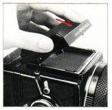
B. To attach the finder on the body, first, simply place protrusions on the bottom of the finder into corresponding openings in the finder frame and, then, slide the finder forward where it will lock.
