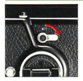
A. To make multiple exposures, rotate the film winding crank (to advance the film and cock the shutter) and then turn the multiple exposure lever in the clockwise or arrow-indicated direction, which will expose a red mark. When set in this manner, the shutter can be released and cocked any number of times, without advancing the film.
