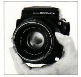
B. All Bronica interchangeable lenses for the ETRS have fully automatic lens diaphragms which means that the focusing screen is always viewed at the full aperture, with the brightest possible image. However, depressing the depth of field preview lever will stop the lens diaphragm down to the preselected lens opening (aperture), permitting the photographer to check the depth of field effect on the focusing screen.
