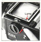
If a red-colored battery check lamp lights up in the left-rear corner (of the waist-level finder) when the battery check button is pressed, the battery is loaded properly and there is sufficient power for electronic operations. \* If the lamp does not light up, (1) the battery is not loaded properly or (2) it is completely drained.
