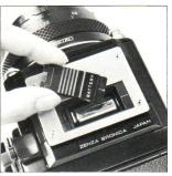
C. Coincide the plus (+) and minus (-) marks on the battery with similiar polarity indications in the battery chamber. Then, push in the negative end of the battery first and follow with the positive end.
