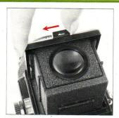
B. To close the focusing hood, first, push down the magnifier (if it is flipped up). Next, press in both side frames, as illustrated, and, at the same time, press the front frame back towards the rear end. The focusing hood will automatically be folded down.
