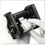
A. After the 15th exposure of the 120 roll film (30th exposure of the 220 roll film), the film winding crank will turn freely with further rotations. Therefore, continue rotating the film winding crank until the remaining film and all the leader paper is wound up on the take-up spool.
