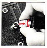
B. Detaching the Strap Simply pull back the plastic catch and revolve 90°, which will leave it locked open, making it a very simple matter to unhook the strap from the eyelet.
