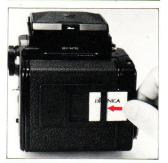
Upon loading the film, tear off the end flap from the empty film package and insert it in the film type indicator frame. This will help you keep track of the film loaded in the film back and should prove useful when two or more film backs are used, with different types of films.
