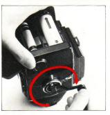
G. The film can be loaded in the film holder, without detachment from the camera body, and should be loaded in the same manner as explained for the detached film holder.
