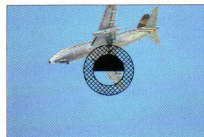
Conventional Split-image Rangefinder
