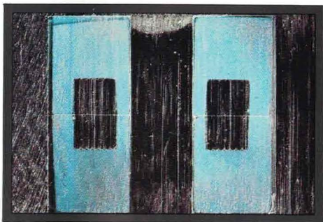
Figure 11: Tape recorder head showing abrasions (X7). A single intense side-light was used to high-light the groove pattern and quantity.
