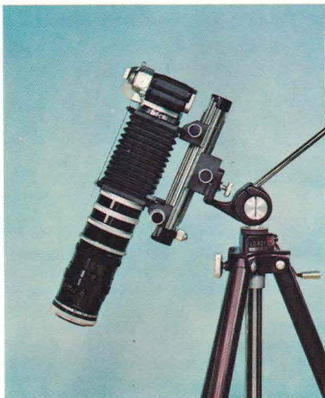
Figure 5: Typical set-up for outdoors; camera body, lens reversed on Macro Photo Coupler, Bellows FL, extension tubes, sturdy tripod.
