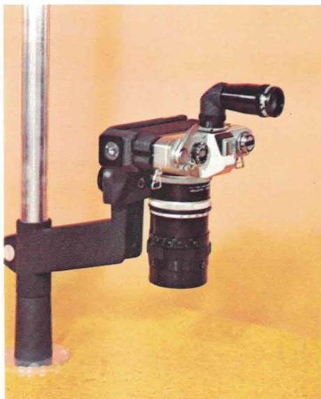
Figure 1: Set-up for same-size photomacrography; Canon FT-QL body, Macro Lens with 1:1 Adapter, Waist-Level Viewer, Copy Stand 3F.
