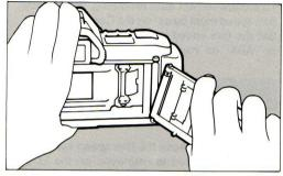
2) To attach the Command Back, insert its lower hinge into the lower socket first. Then depress the hinge release pin, align it with the upper socket and let go off the hinge release pin to lock it on.
