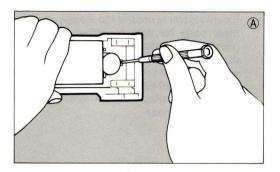
When the "\infty" mark appears to the right of "BATTERY" on the Command Back, the battery has become exhausted. At this time, replace the battery promptly as instructed below.
