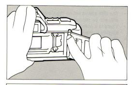
Be sure that there is no film in the camera before attaching the Command Back. Otherwise, the film will be exposed when the regular camera back is opened.
