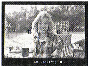
Partial metering circle
