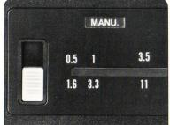
ASA film speed. When ASA 100 film is used, for instance, the upper position is f/2.8 and the middle position is f/5.6.
