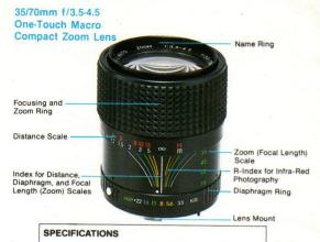
Aperture Range: f3.5-f22 Min/Max. Focus Dist.: 0.4M to infinity Angle of view: 63°-33.5° Elements: 9 groups 9-elements Filter size: 55mm screw-in
