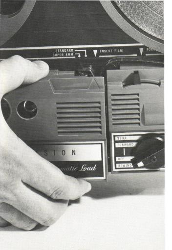
**DAMAGED FILM:** For trouble-free projection, your film must be in good condition. Cut out bad sections of film which have torn perforations, and make certain all splices are aligned and in good condition. Repair poor splices before showing movies to your audience. Film which does not feed through the projector because its perforations are torn or damaged must be removed from the projector for repair.
