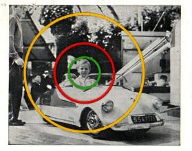
The TELE Attachment enables vou to reduce the normal (30°) measuring angle of your LUNA-PRO either to 15° or even 7.5°. The built-in reflex viewfinder shows you the area to be measured. The illustration at the left shows the three measuring fields of your LUNA-PRO, viewed from the same distance. (The yellow circle which delineates the full 30° measuring field is, of course, not in the viewfinder).
