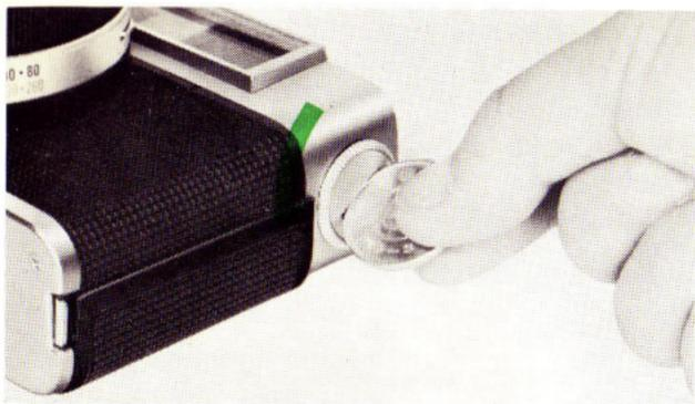
The **KONICA EE-matic Deluxe F's** CdS meter uses a mercury battery as its electric source. Thoroughly wipe the battery, which comes in as an accessory to the camera, with a piece of clean cloth before it is put into the mercury battery chamber.
