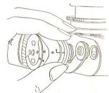
To take the Leica Meter MC off the camera turn the knurled knob into position "B," i.e. as far as it will go. Then pu
