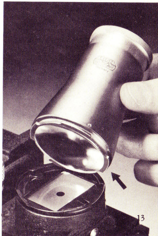
Figure 10. The large wide field magnifier is similarly fitted to the bayonet catches.
