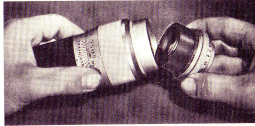
Figure 32. Removing the Hektor 135mm. lens assembly from the mount.
