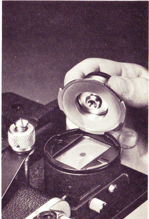
Figure 8. The 30x Magnifier over the clear center spot of the focusing screen, for observation of aerial images.
