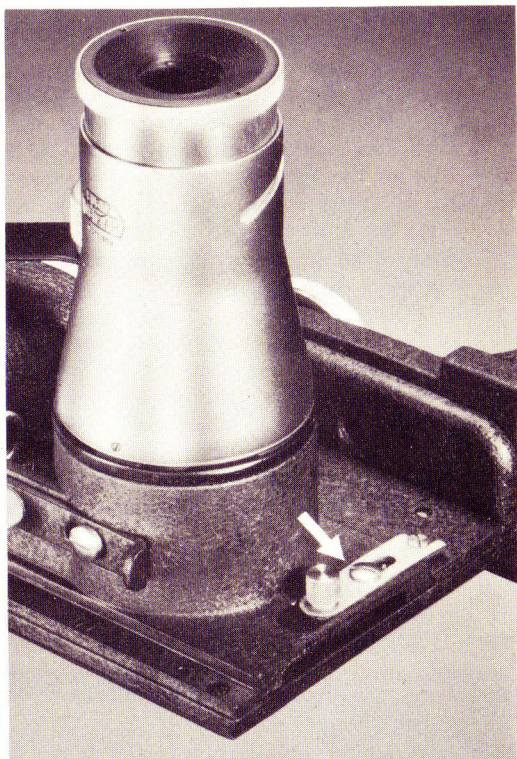
Figure 12. Locking lever at full back position for focusing.
