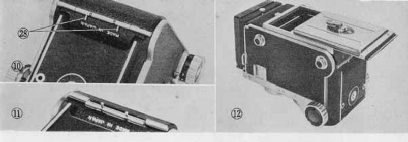
ends of the backlid hinge pivots (28). Lock pivots by turning up into the slots. Backlid (15) then will slide off easily (Figs. 10 and 11).
