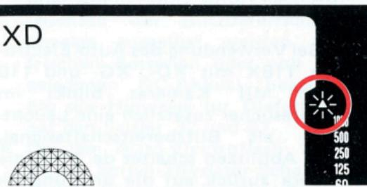
When the Auto Electroflash 118X used with a Minolta XD, XG or 110 Zoom Mark II camera, a flash-ready signal in the camera's viewfinder will blink to indicate that the flash has recycled. After it flashes the 118X will switch the camera back to the previously set mode until it has recycled and the signal starts to blink again.
