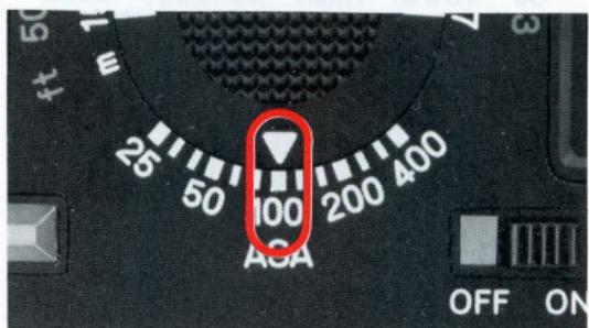
Turn the computer dial to align the exposure-rating number of the film you are using with the triangular white index. (Marks between numbers on the film-speed scale represent ASA ratings of 32, 40, 64, 80, 125, 160, 250, 320, respectively from left to right.)
