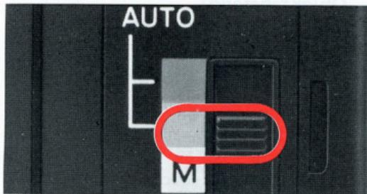
1. With the mode selector at either red or yellow "AUTO" settings, move the power switch to "ON".
