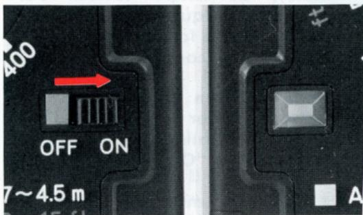
To turn the unit on and charge its capacitor with alkaline, sealed carbon-zinc or Ni-Cd batteries, move power switch to "ON."
