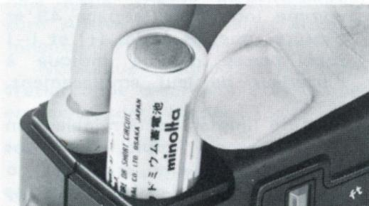
2. After wiping terminals with a clean, dry cloth, insert two carbon-zinc, alkaline or Ni-Cd batteries as specified on p. 43, making sure that plus (+) and minus (-) ends are positioned as indicated inside the chamber.
