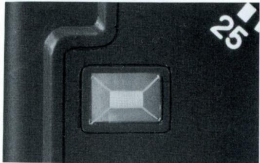
3. With the monitor lamp glowing or the XD, XG or 110 Zoom Mark II camera's flash-ready signal blinking (p. 21), release the camera shutter to take the picture. The Auto Electroflash 118X will automatically vary flash duration from 1/40,000 to 1/3,000 sec. for proper exposure with average conditions and subjects between maximum and minimum flash-to-subject distances.
