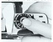
winder will advance the film after each one at a rate of up to two frames per second. In either single-frame or continuous operation, the pilot light will come on during each advance cycle.
