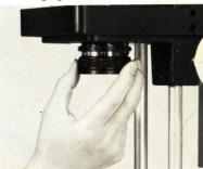
To install the carriage assembly on the column, lower the carriage carefully over the column so that the front and rear rails of the column will fit within the bearings in the carriage shaftway.
