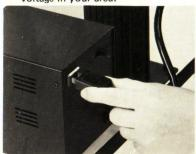
10. The enlarger power supply may now be plugged in to a convenient power receptacle, or into the output socket of a darkroom timer that is itself plugged into a power line.
