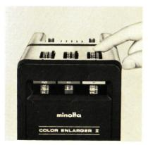
The Color Enlarger II is also a fine black-and-white enlarger. Its diffusion-type light source is the same kind used by most labs and professional printers because of its ability to suppress dust and scratches on negatives. This reduces the amount of time you will have to spend spotting or reprinting. Since you will probably not be using the enlarger's filtration system, make sure all the filter dials are set at their zero position.
