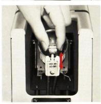
For lamp replacement in the European model, lift the lamp and ceramic socket straight up and out of the retaining clip. Pull the burned-out lamp straight out of the socket. Push the base pins of the replacement lamp into the holes in the socket firmly, as far as they will go. Push straight so as not to bend or break the pins. Carefully slide the lamp and ceramic socket into the retaining clip as far as it will go.
