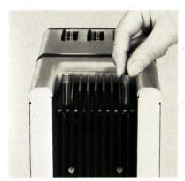
The halogen lamp used by the Minolta Color Enlarger II provides constant brightness and color temperature throughout its working life. When lamp failure makes replacement necessary, first check to make sure that the enlarger's power cord is unplugged. If the enlarger has been in use, wait until the head has cooled before proceeding.
