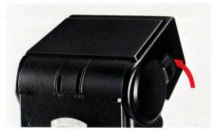
With the Auto Electroflash 28, make sure that the unit is set for automatic mode. With the model 32, set the computer dial for the larger of the apertures available (with the camera lens set to the same f-number), this is advisable since the comparative strength of light falling on the subject is considerably reduced with bounce flash, the exact amount varying widely with bounce conditions.
