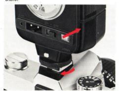
With other cameras, secure the bracket in the accessory or flashgun shoe in the same way; insert the single-prong plug on one end of the attachable sync.-cord provided into the flashgun's sync.-cord socket until it snaps in place; and plug the PC connection on the other end into the camera terminal for "X" synchronization.
