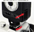
2 Set applicable film speed on computer dial of flash unit (p. 10).
