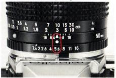
4. With the monitor lamp glowing, release the camera shutter to take the picture. The unit will automatically vary flash duration from 1/40,000 to 1/1,000 sec. for proper exposure with average conditions and subjects between maximum and minimum flash-tosubject distances.
