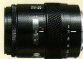
MAXXUM AF 35-105mm f/3.5-4.5 Minimum focus (macro): 4.9 ft. (1.3 ft.) Maximum magnification: 0.25X Filter-mount diameter: \phi 55mm Dimensions: \phi 2-11/16 \times 3-7/16 in. Weight: 1 lb. 1-1/8 oz.
