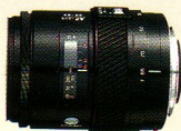
MAXXUM AF 28-85mm f/3.5-4.5 Minimum focus (macro): 2.6 ft. (0.8 ft.) Maximum magnification: 0.25X Filter-mount diameter: \phi 55mm Dimensions: \phi 2-11/16 \times 3-3/8 in. Weight: 1 lb. 1-15/16 oz.
