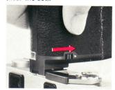
Removing unit from camera automatically switches the unit off. The manual switch should be set in the off position (away from the dot) to conserve batteries whenever the unit is attached to the camera but you are not taking pictures.
