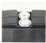
Replace cover by aligning carefully, depressing ends of batteries slightly with it, and sliding it toward guide-numbertable side of unit until securely in place.
