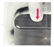
2. Insert two batteries (see specs. p. 1), making sure that plus (+) and minus (-) ends of batteries are positioned as indicated inside battery compartment.
