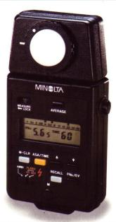
Multi-purspose exposure meter for incident/ reflected flash/continuous light with liquid-crystal digital-analog readout and memory.
