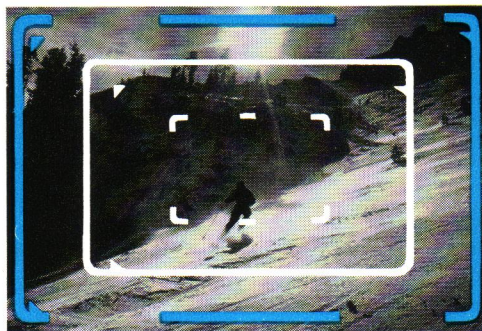
Subject seen through Trifocal Finder: full frame represents 35mm field of view; middle frame for 50mm (normal) lens; inner-most frame for 105mm telephoto.
