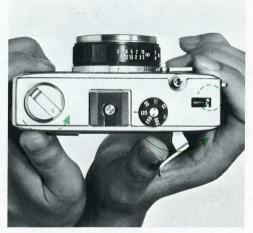
Advance film by rotating film advance lever and depressing shutter release button alternately until No. 1 appears in film exposure counter window on top of camera.
