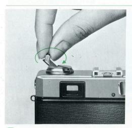
Make certain sprocket wheel engages in perforation in film properly before closing rear cover. Close rear cover click.
