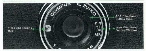
Depress ASA ring in the front of camera slightly and rotate it around the lens to select ASA (or DIN) rating for your film. For perfect exposures, the correct ASA or DIN film speed of your film must appear in the ASA setting window. The window is in the right side of the lens as viewed from frontward.
