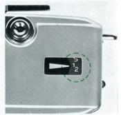
The film counter shows S, 1, 2, 4 and subsequent even numbers up to 36. The numbers 12, 20 and 36 are in yellow color. Each time the film is advanced, the counter counts up the number of exposures made, which is pointed by the orange color arrow (). When the rear cover is opened, the counter returns automatically to S.
