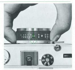
Turn F/stop ring to bring the mark ( & ) to the center index on the lens barrel. If the mark "A" is set to the center, shutter release button might be locked, blocking smooth loading when you load in a dark place.
