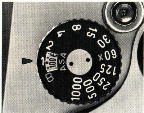
The ASA film speed rating of all 35mm films is given in the data sheet packed with each roll of film. The higher the ASA number, the more sensitive the film. Lift the outer ring of the shutter speed dial and rotate it until the ASA number of your film is opposite the orange dot alongside the figure 1.
