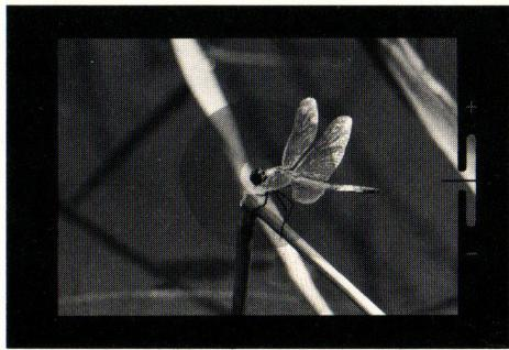
The microprism is the center portion of this diagram. When your subject is in focus, the image in the microprism will be sharp and perfectly clear. If your subject is not in focus, the microprism will break the image into many small dots, much like an engraver's screen. You can focus your subject on any portion of the ground glass.
