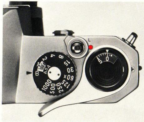
With the shutter speed dial set on B (bulb), the shutter will stay open as long as you depress the shutter button. As you release your finger from the shutter button, the shutter closes. When a long exposure is desired while using the B setting, set the shutter button lock by moving the lever to the left (an "L" becomes visible) while depressing the shutter button. Alternately, use a cable release with a locking device. This will permit a "Time" exposure.
