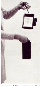
4. Pull the yellow tab all the way out of the camera: Pull straight, smoothly, at medium speed, without slowing down or stopping. Pull the camera up with your left hand as you pull the tab down with your right hand.
