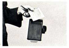
2. Pull the white tab out, but before pulling the yellow tab take out the warmed Cold-Clip and hold it as shown. 3. Pull the yellow tab out of the camera.
