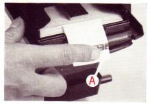
1. Unlock the back of the camera, open it part way and, without disturbing or moving the film pack, push the white tab (A) out into the open.
