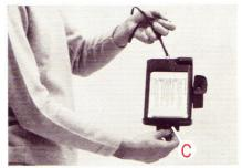
7. Pull the safety cover all the way out of the camera: Pull it straight and be careful not to rip it.
