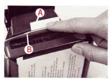
2. Close and lock the back of the camera, making sure that the white tab (A) is outside and behind the lock (B).
