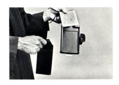
4. Immediately open the Cold-Clip and place the entire piece of film inside the Cold-Clip with the tab hanging out as shown. This must be done within 10 seconds after pulling the tab out.
