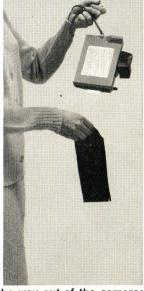
4. Pull the yellow tab all the way out of the camera: Pull it straight, smoothly, at medium speed, without slowing down or stopping. Pull the camera up with your left hand as you pull the tab down with your right hand.
