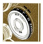
In special cases (flash, high filter compensating numbers over -3) the filter is compensated for by decreasing the film speed by 3° DIN for each full value (for example, when working with Neutral Density filter No.  $4:-4=4\cdot3^\circ=$  requires setting the meter to  $12^\circ$  DIN less than the actual film speed).
