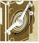
Adjusting to DIN / ASA speed ratings ①: First determine the speed of the film used (to be found on the box or an accompanying instruction sheet), which will be indicated in DIN or ASA values. Gently press and turn knurled knob until the corresponding speed rating appears above the indicator mark in the DIN or ASA window. (The dots correspond to intermediate film speeds, → page 27.)
