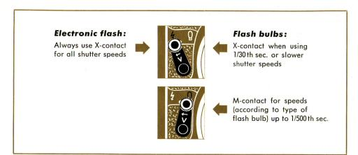
The correct exposure depends on the light output of the flash and the distance between flash and subject. Therefore, it cannot be determined with an exposure meter. Exact data regarding choice of proper contact, exposure time and diaphragm may be gathered from the material furnished by the lamp manufacturers.
