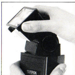
2. To adjust the Flash Base, simply twist as illustrated with thumb and forefinger.
