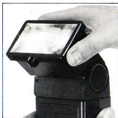
1. To rotate the Adjustable Bounce Flash Head, grip with thumb and forefinger and gently turn to the desired setting. DO NOT FORCE THE HEAD.
