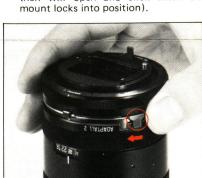
C. Slide the coupling key of the mount into the matching slot of the lens aperture ring. Sometimes the coupling key will slide into the matching slot after step B and therefore this step may not
