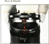
B. Press the mount downward and turn clockwise until the mount is locked into place (while turning, the silver release button will slowly depress and then will open and click when the mount lock into position)
