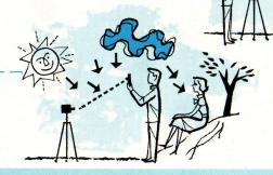
Reflected light is light reflected from the subject to the camera. Incident light is the light which falls on the subject. Measurement of either reflected or incident light can be used to determine correct exposure.
