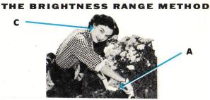
Hold the meter as shown on page 7 aiming toward the scene from the camera position. Point the meter down slightly to avoid reading sky areas which will give inflated values and cause underexposure. Set the arrow on the exposure control dial to the light reading obtained, for example 400.
