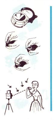
Your meter can be converted to read incident light simply by attaching the Weston Invercone. The Invercone consists of an Integrating Cone and an Auxiliary Multiplier.
