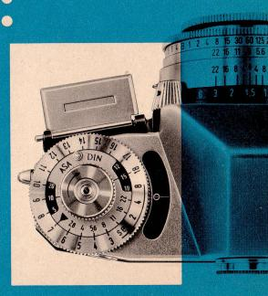
On the CONTAFLEX II the meter shows aperture and shutter speed, on the CONTAFLEX IV the exposure-value, because the models III and IV have exposure-value shutters with coupled shutter speed and aperture settings. These shutters also have a lock to prevent accidental alteration of the flash setting lever.
