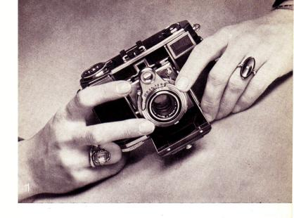
If you now turn the lens focusing ring(6) (see illustration above) until the two images merge into one (see illustration on preceding page, lower right), the lens will be accurately focused. The best objects for obtaining accurate focus are sharply defined vertical contours. Precise focusing is the more essential the greater the lens opening.
